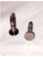
Next in the Kohler build-up is the valve train. The springs, retainers, keepers, and valves are stock Kohler parts. I used the more expensive Stellite exhaust valve, P/N 235838 for good durability.
