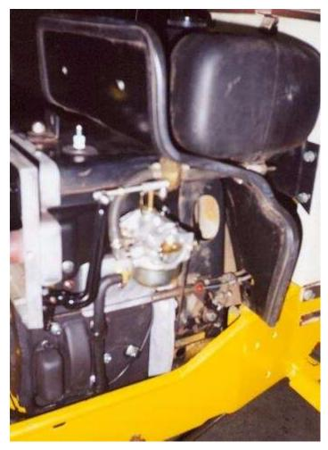
This shows the right side of the engine where the Mercury outboard voltage regulator replaces the stock item. This contains the tach driver circuitry for the instrument panelmounted Datcon tachometer. The chrome coil is an aftermarket unit made by Compu-Fire.
