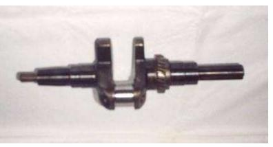
losses but more importantly, a smooth surface is less prone to fail due to reduced stress concentrators. After polishing, a coat of Hoppe's gun bluing was applied to make it look nice and prevent rusting. The crankpin was left un-blued, but polished with 600-grit emery cloth (lightly).
