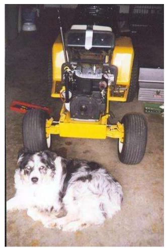
Mac guards the treasure! Here the engine is bolted in and we're getting close to the first run. During this time, the tractor engine bay was thoroughly cleaned and new rubber mounts were installed on the engine mounting rails. The PTO clutch was also inspected and cleaned.
