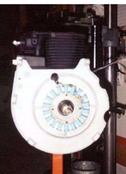
Here the oil pan, dipstick tube, and head are bolted on and carefully torqued to book specs. I know it's anal, but I paint both sides of the flywheel (after masking off the magnets). Don't like the thought of bare iron rusting!
