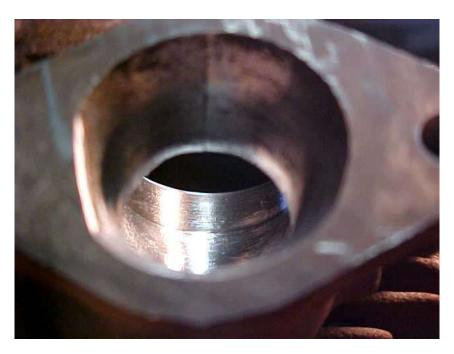
The exhaust port gets the same treatment, although not as extensive. Removing sharp corners and blending are performed here.
