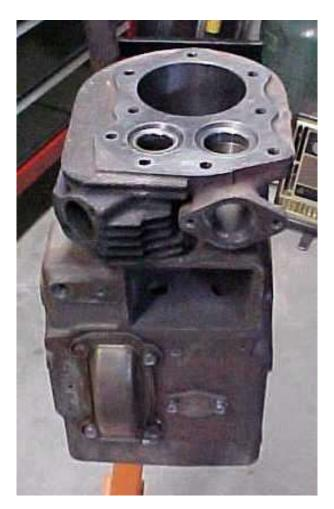
The deck was first to get some grinding work. The stock valve pockets are machined in from the deck face and have rather sharp edges for gas flow to traverse. This is what the stock deck surface looks like.
