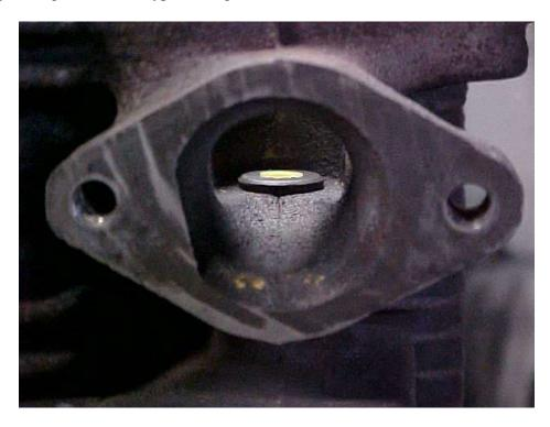
Some careful grinding using medium grit stones and emery flapper wheel smoothes out the surface and allows a flow improvement. A mirror finish is not necessary, but just smooth to the touch.
