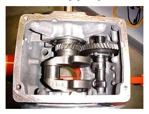
The bearing plate was then fitted using one black and one brown gasket, and bolts torqued to 35 foot pounds. Note new grade 5 bolts fitted. Crank end clearance was checked and found to be .005 in., right in tolerance range.
