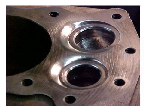
The intake and exhaust ports are next. The stock intake port is formed by a sand core during casting and has the typical rough surface found on cast iron blocks.
