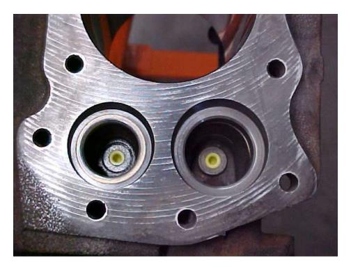
Blending these edges and taking out all sharp corners is known as a "relief". The modification increases volumetric efficiency by creating less restriction to gas flow. This is a partial relief, as pockets are blended into the existing deck face. A full relief extends a full depth cut all the way to the bore circumference. The material is not very thick on the block casting in this area thus I'm leery of doing full reliefs on Kohler engines.
