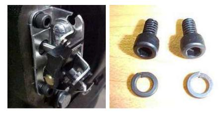
Screw size is  $\#10-24 \times 3/8$  and four are required – two for the points and two for the cover.
