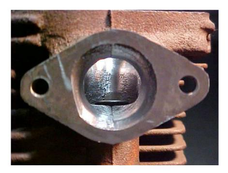
The inside radius of the port is a very important area to blend. Some blocks have rather sharp corners here that need to be blended into a smooth continuous radius
