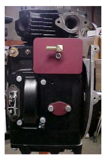
The cylinder head was bead blasted and cleaned up nicely.
