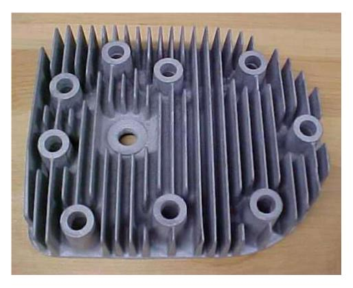
The sealing surface was decked .025 in the mill to raise compression ratio slightly.
