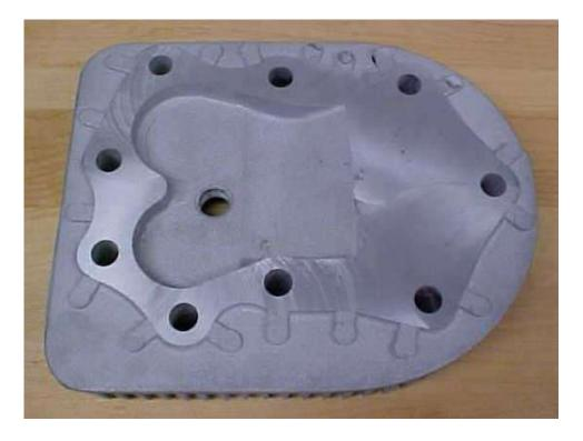
Prior to fitting the head to the block, all bolt holes were chased with a well-oiled tap. This assures accurate torque values.
